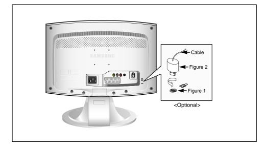
The Kensington lock is a device used to physically fix the system when using it in a public place. The locking device has to be purchased separately. The appearance and locking method may differ from the illustration depending on the manufacturer. Please refer to the manual provided with the Kensington lock for proper use.
